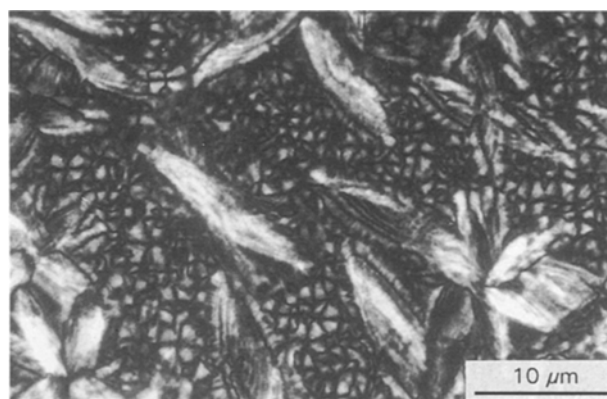
Figure 6 Optical micrograph of polymer PE-4 isothermally crystallized at 122°C and subsequently cooled to room temperature.
